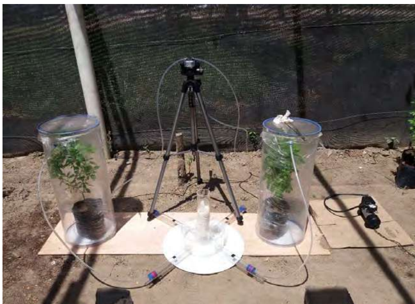
Figure 1. Olfactometer adapted with two chambers to study the interaction between Tetragonisca angustula , Ocimum basilicum , and the microorganisms associated with O. basilicum .
